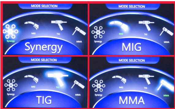
Easy selection between Synergy, MIG, TIG and MMA mode
